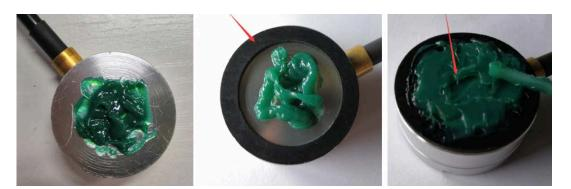
Insert the sensor into the holder and install the cover plate.
