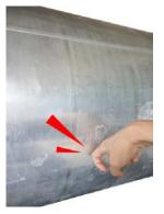
When there is fuel in the fuel tank, you can hear a muffled sound.
