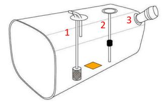
If the fuel tank is cylindrical, choose the area that is closest to the ground such as the section shown in the following figure.
