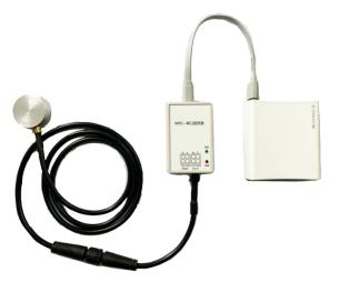
3) Turn on the list of available wireless networks on your mobile phone, select the network which start with <u>USR-WIFI</u> and click connect. Once connected, the green indicator light is on.
