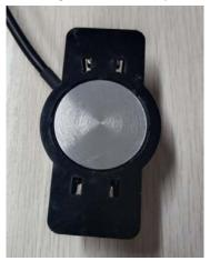
Stick the probe on the marked location and check the app result is ok or invalid. If no, move the probe slowly within 2–3 mm and find the right installation location.
