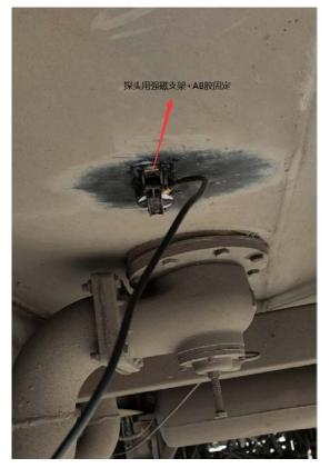
If the ambient temperature is 25°C, move the probe for 30 seconds after sticking the probe. In this way, if the result is unable to install, remove the probe, clean up all AB glue, and apply glue to the probe surface again. Because the AB glue does not work at this moment.
