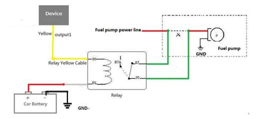
Note: To implement remote fuel/power cut-off, connect the relay to the fuel pump power cable or to the engine power cable in series.
